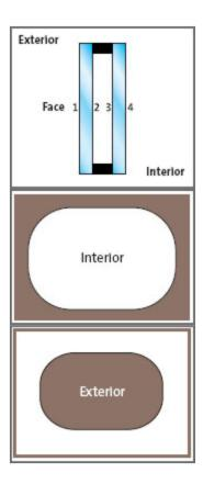
Condensation forms very differently depending on whether it is inside or outside the building, due to the thermal bridge effect around the cavity.
