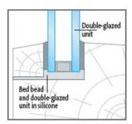
These are known as drained and ventilated systems. They can be applied to most types of frame including aluminium, PVC-U, steel and timber.
