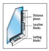
The number and spacing of the blocks relates to the size of glass pane, framing system and conditions of use.
