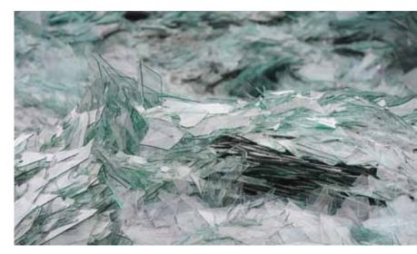
On average 30% of the total weight of a sheet of glass made by Saint-Gobain Glass comes from recycled internal cullet and "pre-customer" cullet.
