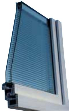
*In a ScreenLine® system, the blind (venetian, pleated or roller) is encapsulated within two glass panes, e.g. in a double glazing unit. The movement of the blind, for manual or motorised systems, does not compromise the insulating properties of the D.G. unit, and therefore operates in a totally sealed environment.*
