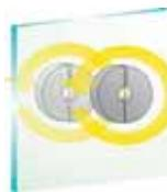
[ The ScreenLine® system designed with the rotational frontal magnetic control, for raising and tilting a blind integrated within a double-glazed unit, utilises the force produced by two coupled rotational magnetic devices. One set of magnets is inserted in the blind head rail within the cavity and the other applied to the external glass surface. This magnet principle does not
