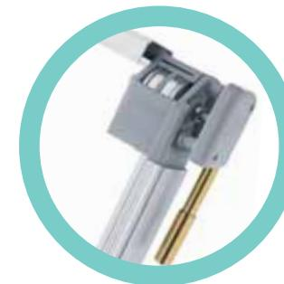
[ *The ScreenLine® SL20P system comprises a venetian blind incorporating a 12.5 mm slat designed to be integrated in a double-glazing unit with a 20 mm. cavity. The manual tilt only function is operated via a wire drive by an external knob. The specially designed corner key containing the rotational magnet is connected to the external knob by a flexible drive cable located within the glazing cavity of the*
